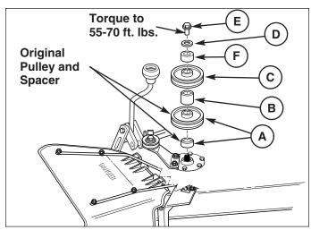
Figure 10. Install Turbo Drive Pulley
